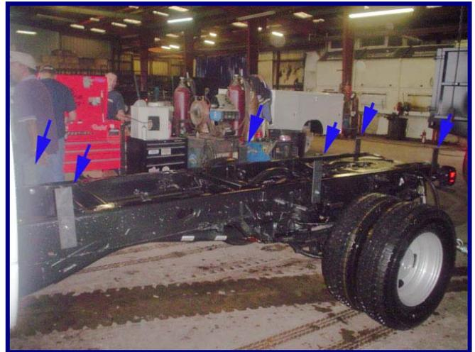
2. Install the straps using the supplied 1/2' x 1 1/2" bolts, flat washers, lock washers and nuts. You will find it helpful to install the bolts so the nuts are to the outside of the truck frame. This will make it easy to tighten the nuts and will also make final inspection possible from the outside of the truck frame. Snug bolts just enough to keep the mounting straps standing straight up. Watch for wires, hoses or brake lines inside the frame.
