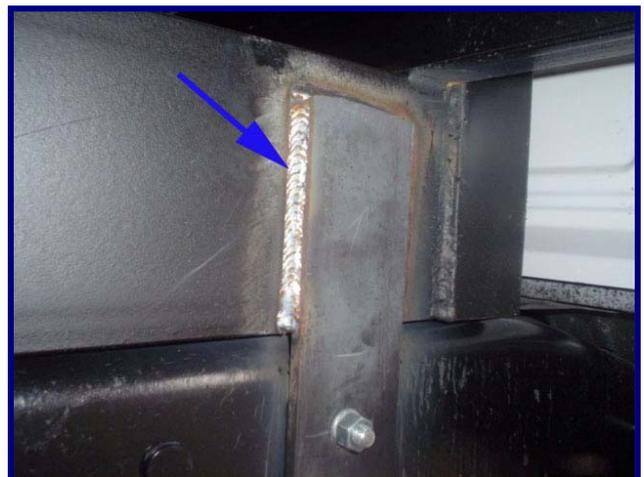
6. Tighten the 1/2” bolts to the truck frame, taking care not to pinch any wire or lines inside the truck frame.
