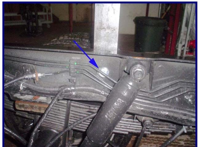
3. Lift the body by lifting from the stake pocket holes taking care not to scratch the paint. Two lifts will be necessary with one pair of spreader chains on each hoist.
