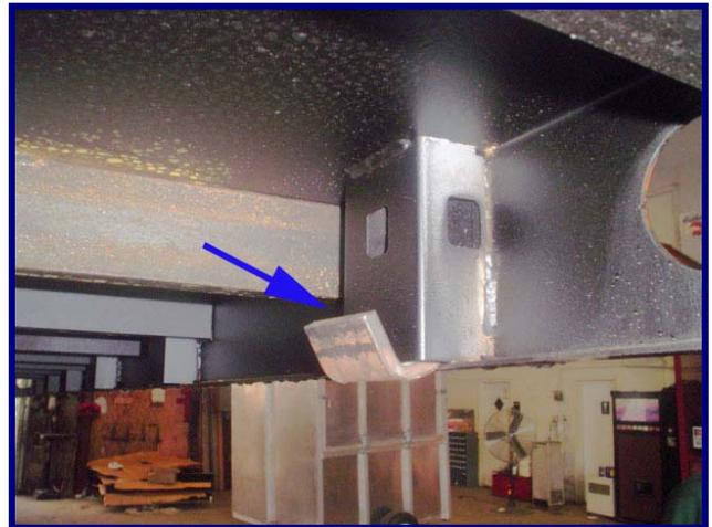
4. Lower body to the truck frame using the body mounting straps as a guide. Body should be set about 3” from the cab. Take care to leave adequate clearance so frame twist doesn’t cause the body to contact the chassis cab.
